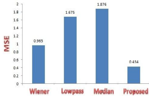
Figure 9. Comparison chart of MSE of different denoising methods for microarray images
