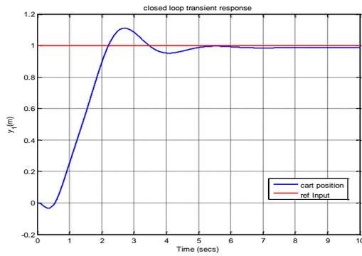
Figure 7 (a) Transient response (Cart Position).
