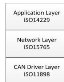
Figure 1. Structure and UDS diagnostic protocol stack
