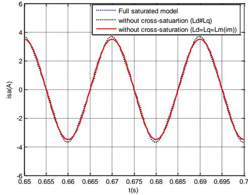
Figure 4. Stator phase current predicted by  $(\bar{i}_s, \bar{\lambda}_s)$  model.
