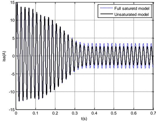
Figure 2. stator phase current predicted by full saturated model and by unsaturated model
