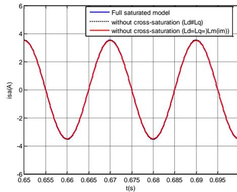
Figure 5. Stator phase current predicted by  $(\bar{i}_s, \bar{\lambda}_r)$  model.
