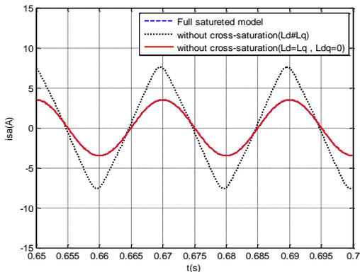
Figure 3. Stator phase current predicted by  $(\bar{i}_s, \bar{i}_r)$  model.
