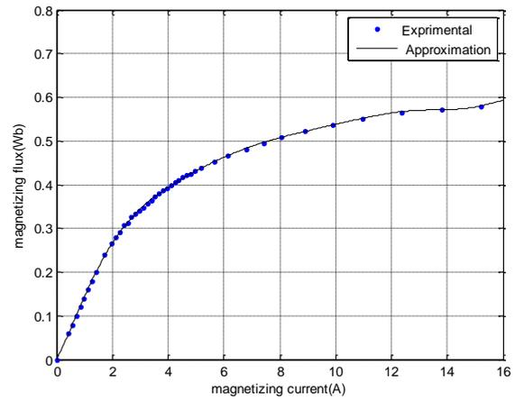
Figure 1. No-load saturation curve for induction machine
