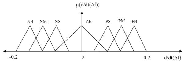
Figure 4. (b) Membership functions of derivative of frequency error (d/dt(Δf))
