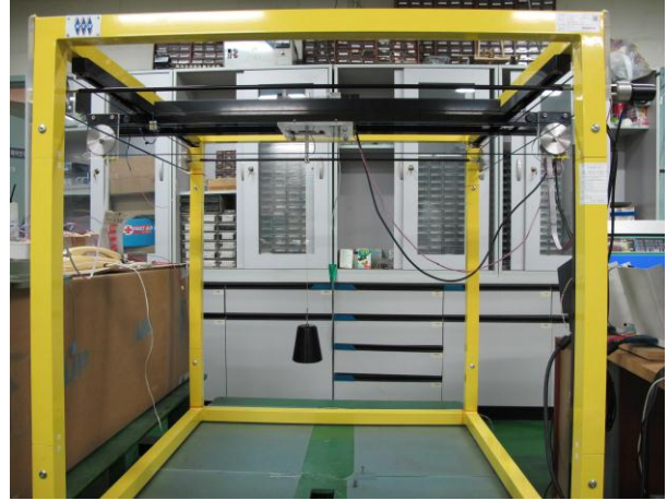
Figure 2. An overhead crane system for experiment
