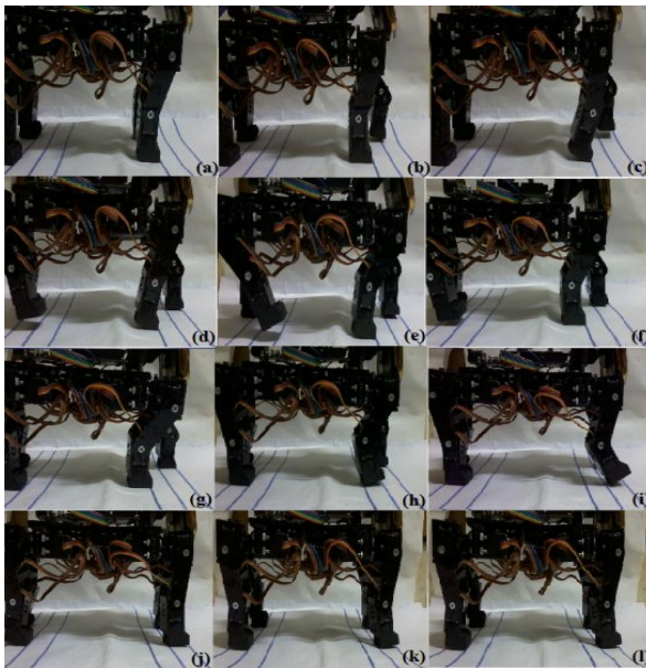
Figure 16. The sequence of the straight-walking obtained.
