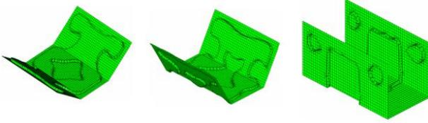
Figure 5. Topography model of the folded plate after optimization with folding angles  $\alpha = 30^\circ, 60^\circ$  and  $90^\circ$
