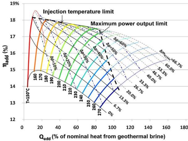
Figure 4. Additional heat conversion efficiencies obtainable by exploiting the additional heat source [35].
