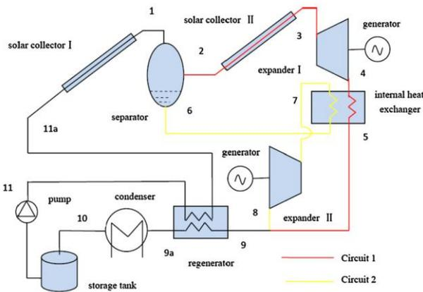
Figure 5. Schematic diagram of ALSRC system [41].
