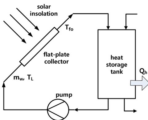
Figure 2. Schematic diagram of the solar collector and thermal storage system.
