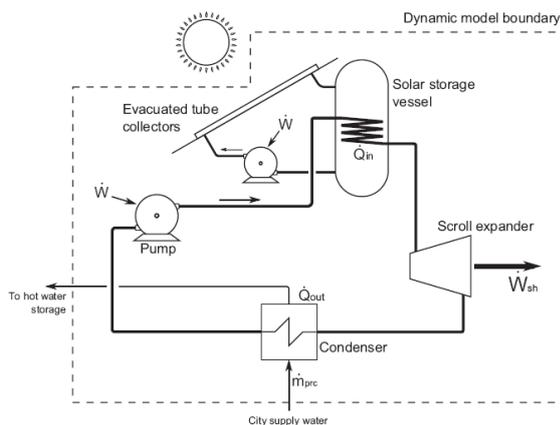
Figure 3. Solar ORC system configuration [30].
