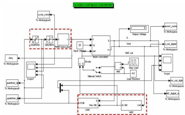
Figure 5. Buck converter digital closed loop Top-Level model
