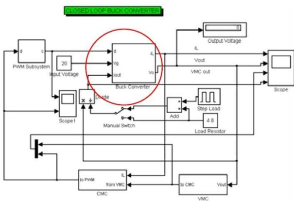
Figure 3. Closed loop buck converter system
