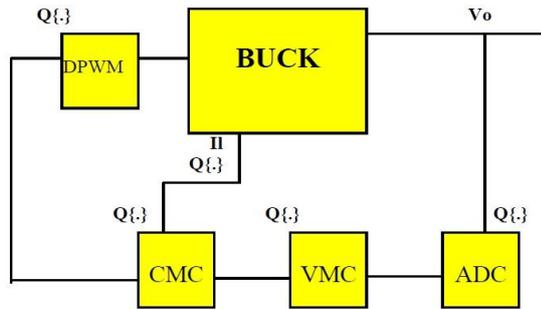
Figure 1. Block diagram of quantization scheme
