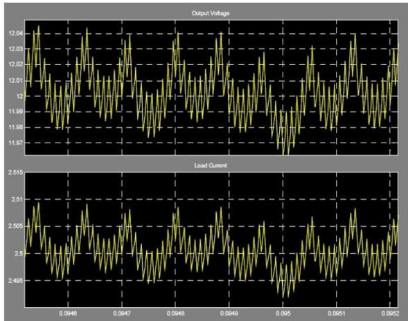
Figure 8. Output voltage response with DPWM quantized to 4-bits
