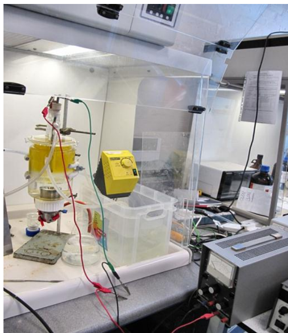
Figure 9. The custom glassware during electrolysis of KOH
