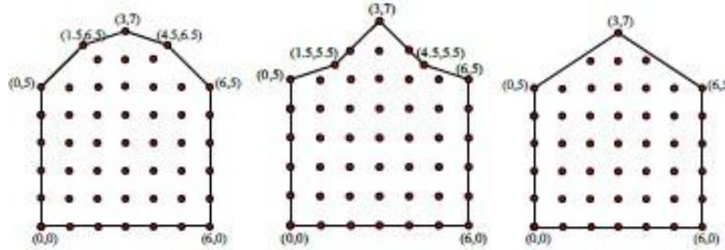
Figure 4. Grid points for finite difference method
