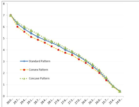
Figure 8. Temperature at centerline of each roof geometry by Finite Element Method
