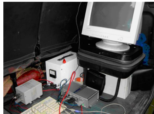
Figure 6. The INS/GPS system in outdoor experimentation
