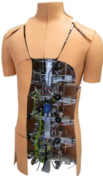
Figure 1. The construction of the male robotic mannequin. The internals of the mannequin can be seen.
