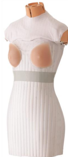
Figure 3. The new cover design and the prosthesis used for breasts of a female robotic mannequin.
