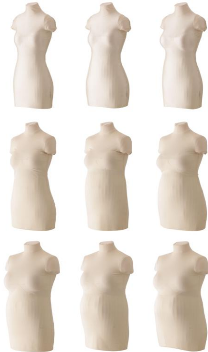
Figure 4. Set of three female robotic mannequins. Each row represents one mannequin in different shapes.
