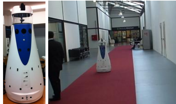
Figure 1. Left: the RobVigil robot equipped with the tilting LRF at top. Right: the robot performing a surveillance routine
